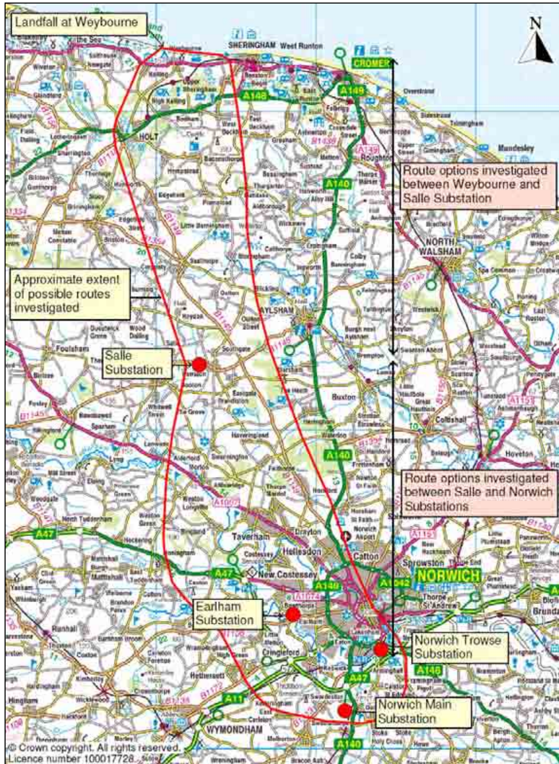
Figure 2.2 Extent of area assessed for possible cable route options during the initial cable route identification studies between Weybourne and Norwich
