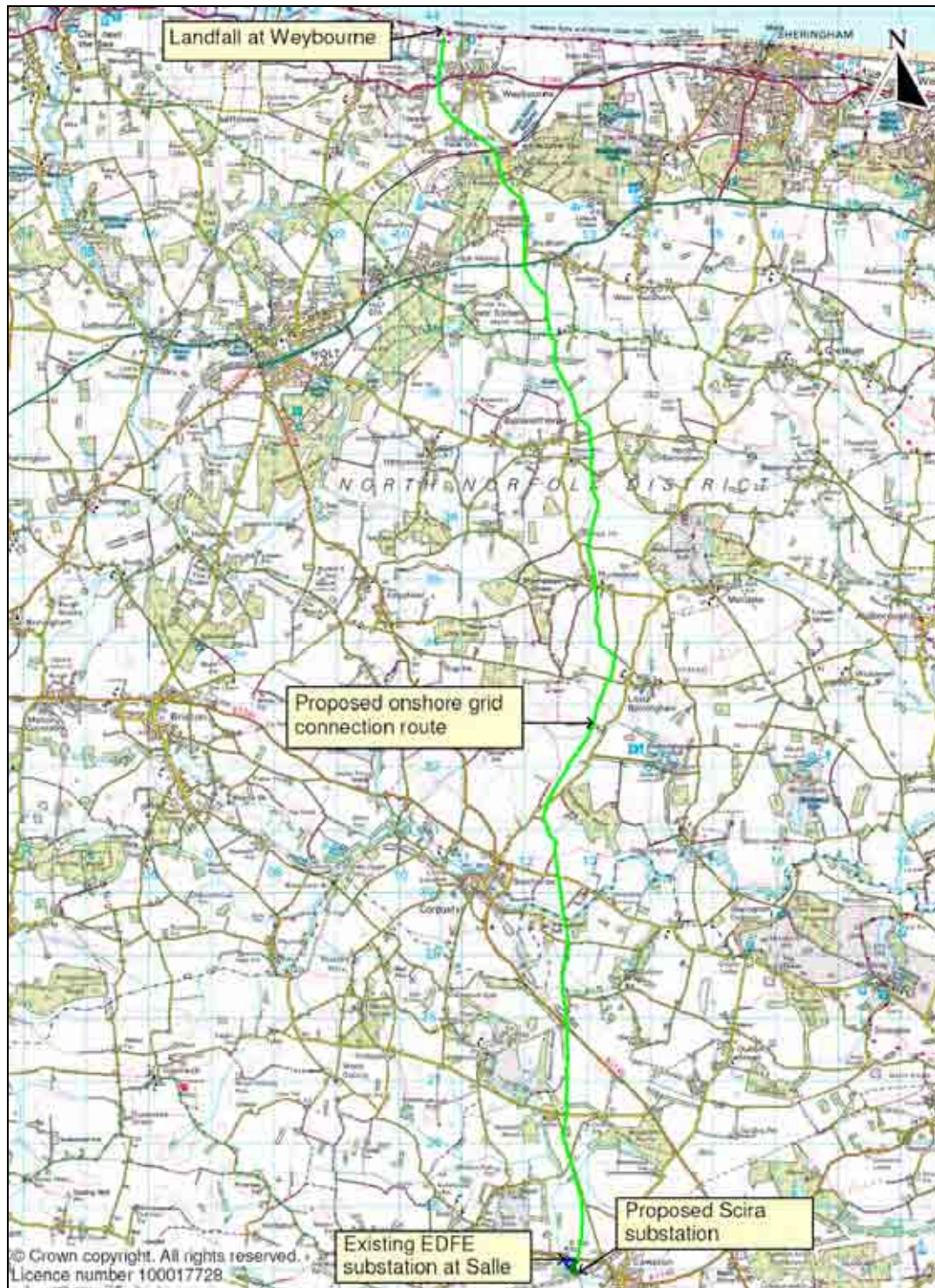
Figure 3.1 Proposed onshore grid connection overview
