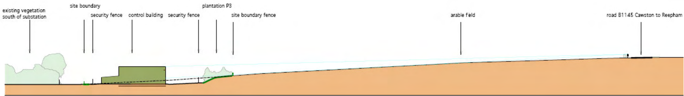
Section between control building and B1145 cawston to Reepham road Vegetation illustrated after 15 to 20 years growth. View lines to building and equipment shown. Extent of cutting shown, building outline simplified (accurate maximum height) scale 1:500
